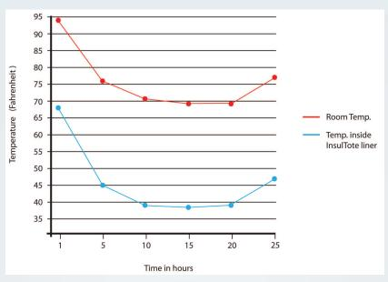
Testing was conducted in a controlled environment using a standard corrugated box lined with an InsulTote insulated box liner. Items placed inside the liner were (12) 4.25 oz. candy bars and (4) coolant bricks.
