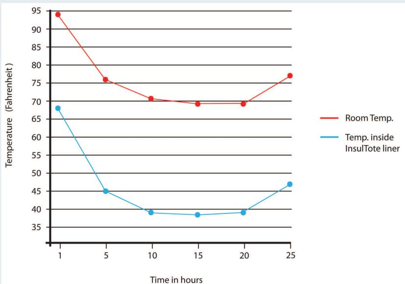
Testing was conducted in a controlled environment using a standard corrugated box lined with an InsulTote insulated box liner. Items placed inside the liner were (12) 4.25 oz. candy bars and (4) coolant bricks.
