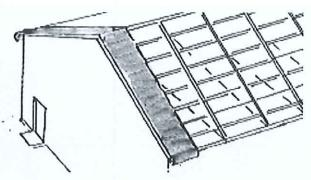
Starting at the end of the roofing framework. measure the length across the trusses, adding enough to allow overhang at both ends. Cut the first piece and lay in place. Pull tight from both ends and attach to trusses or purlins using selftapping screws and washers or with pressuresensitive reflective tape. Cut the second length, laying parallel to first. Make sure to butt or slightly overlap edges. Tape all seams.
